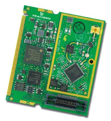
The Tranzeo TR-WMX-5.8-mPCI 5.8GHz Mini-PCI card based on the IEEE802.16-2004 standard is ideal for custom subscriber units and other embedded applications. Tranzeo's family of WiMAX products are based on a WiMAX Forum Certified<sup>™</sup> design to ensure seamless interoperability with all WiMAX Certified<sup>™</sup> systems.
